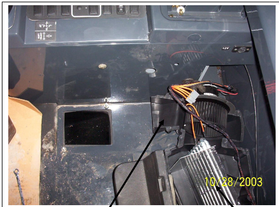
Top half of heater box removed. Top half of blower housing is part of the same assembly.
